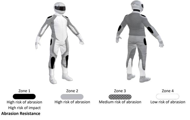
The garment was tested for abrasion resistance in accordance with MotoCAP test protocols. The table below shows the test results for time to abrade through all layers of the materials. Calculated for each sample by Zone, type and area coverage of each material as a proportion of that Zone.
