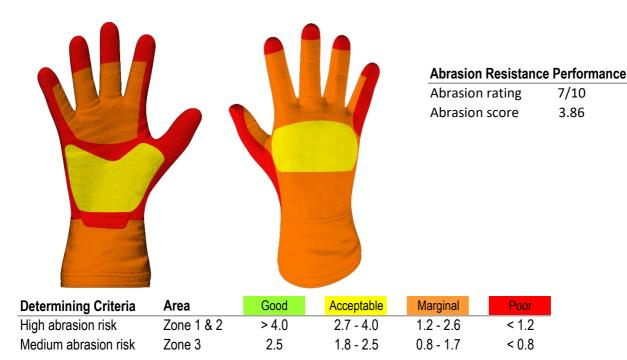
**Individual Abrasion Resistance Results:** - The table below shows the test results for time to abrade through all layers of the materials. Calculated for each sample by Zone, type and area coverage of each material as a proportion of that Zone. Abrasion times are capped at a maximum of 10.00s.
