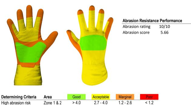
**Individual Abrasion Resistance Results:** - The table below shows the test results for time to abrade through all layers of the materials. Calculated for each sample by Zone, type and area coverage of each material as a proportion of that Zone. Abrasion times are capped at a maximum of 10.00s.
