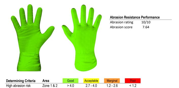
**Individual Abrasion Resistance Results:** - The table below shows the test results for time to abrade through all layers of the materials. Calculated for each sample by Zone, type and area coverage of each material as a proportion of that Zone. Abrasion times are capped at a maximum of 10.00s.
